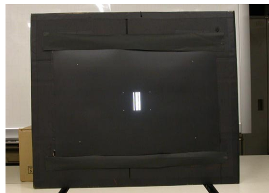
(Fig. 6- Setting board is blackened with the chart being attached.)
