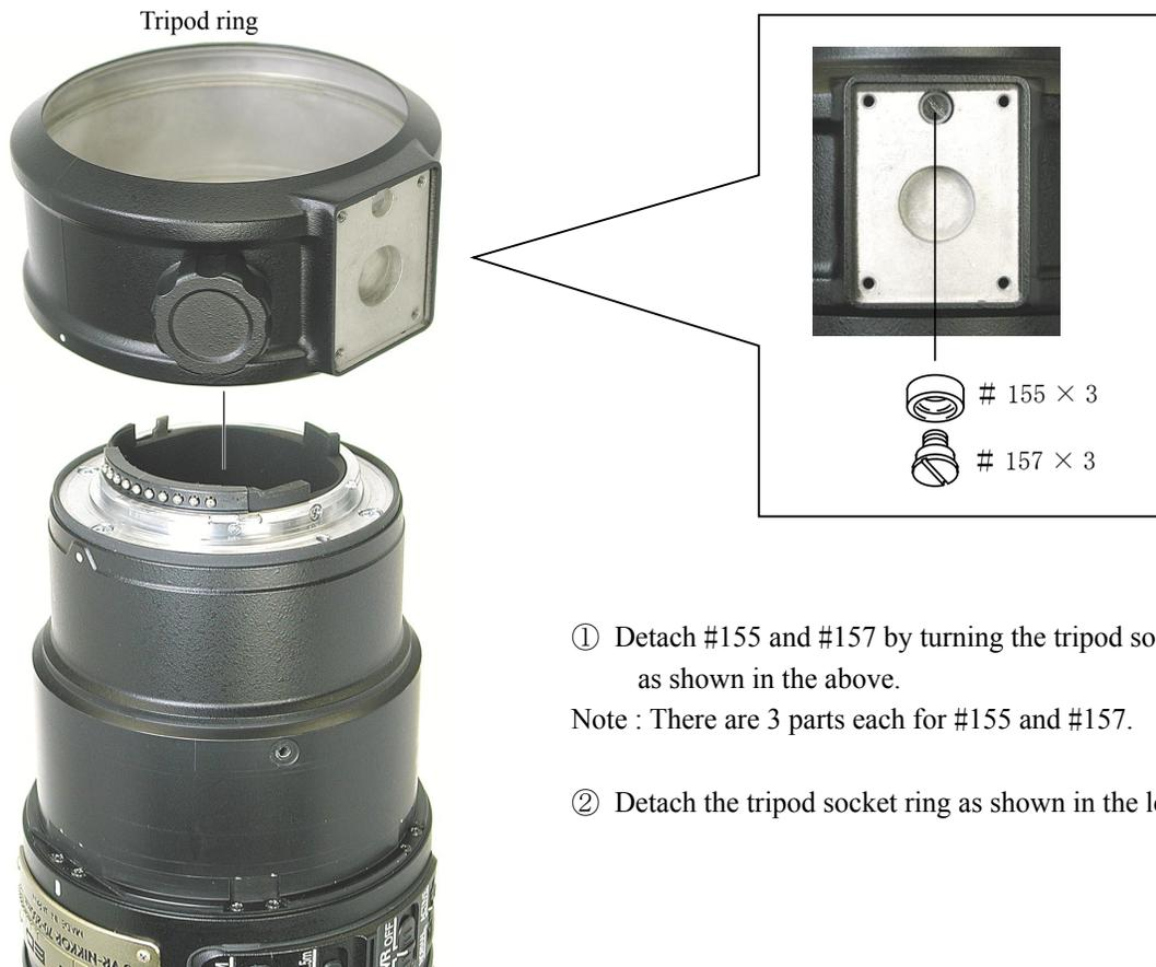
① Detach #155 and #157 by turning the tripod socket ring as shown in the above.
