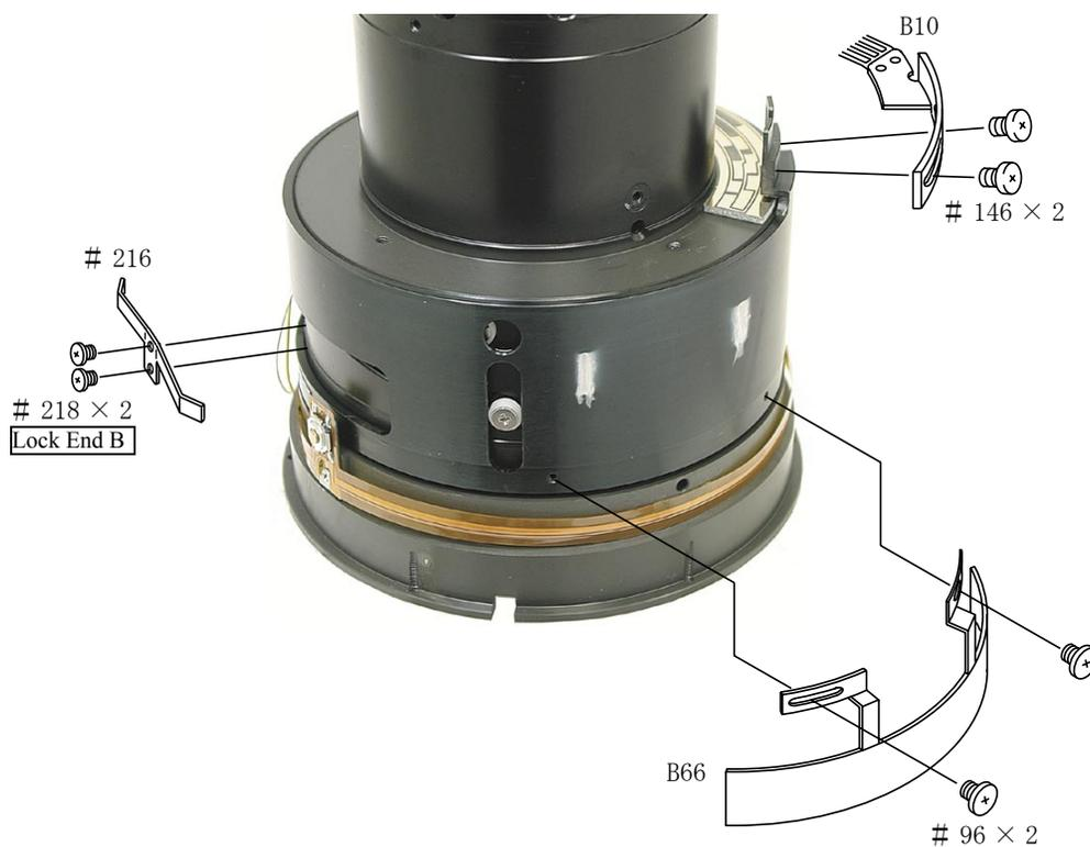
※ Screw temporarily the 2 screws each for #146 and #96.
